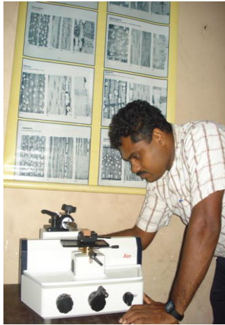
Cutting thin wood section using Microtome
