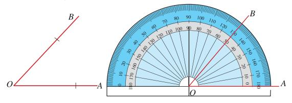
Place the protractor on the figure such that the origin and the base line coincide with the vertex O and the arm OA respectively.
