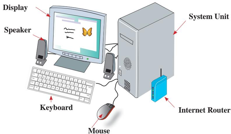
Figure 1.3 - Components of a Computer
