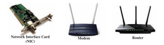
Figure 1.9 - Wired/Wireless Communication Devices
