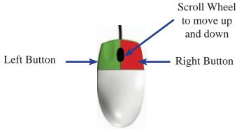
Figure 4.3 - Main Parts of a Mouse
