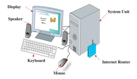
Figure 1.3 - Components of a Computer
