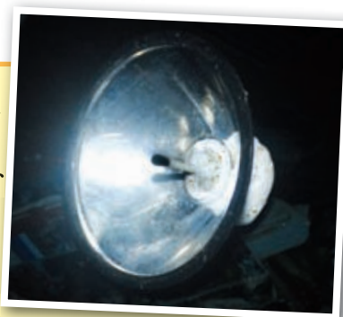
Figure 19.5 ▲ A torch reflector
