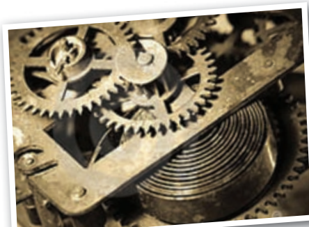
Figure 7.8 ▲ Inside a clock, that works by potential energy stored in a spring
