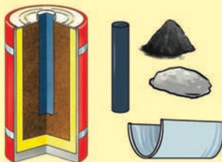
Figure :- 3.2 ▲ Contents of the dry cell
