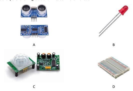
Ultrasonic Waves Sensor, Passive Infrared Sensor(PIR), Light Emitting Diode(LED), Bread Board
