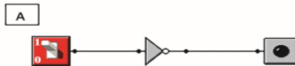
If switch is on(1), the LED bulb will not light up.
